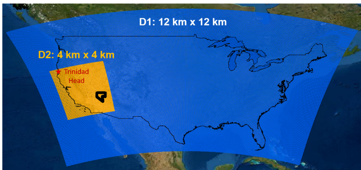
Figure 11-1. Map of WRF-Chem model domains, including of the contiguous US (D1: 12 km x 12 km) that feeds an inner domain (D2: 4 km x 4 km) of the Western US. Trinidad Head ozonesonde launch location denoted by red star.
