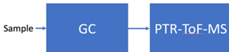
Figure 7-3. Pre-separation allows for identification of interferences and fragmentation patterns.
